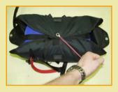
8) Put the packing line (in the Handy kit) through the container loop and close the opposite flaps on the longer side of the container.
