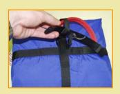
1) Link the handle of the harness with the central loop of the inner reserve container (thread the handle through the loop). You always insert the reserve with the final loops in the above part of the container.
