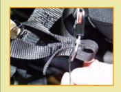
14) Check the details of putting the straps through the small buckle. Please note the way the small "safety" strap is put through the buckle. The safety strap prevents the container on its position even of the buckle is accidently opened.
