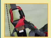
13) Fix the upper part of the container into the main carbine exactly as you see in the picture.
