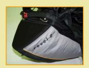
3) Place the risers into the tube on the side of the harness and fix the tube flap by the Velcro.
